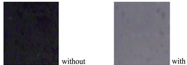
Figure 9 (b) Optical Photo Graph of D.C Sputtered Tantalum Thin Film (177.5nm) with and Without Hydrogen
