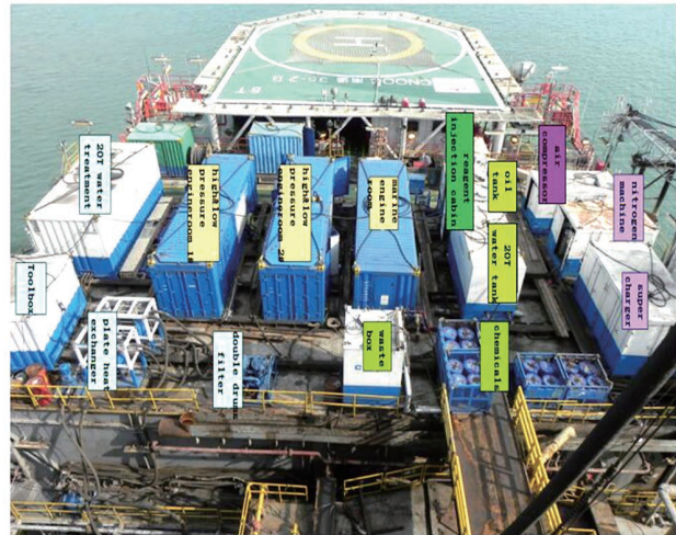
Figure 3 Thermal Recovery Process Based on the Platform
