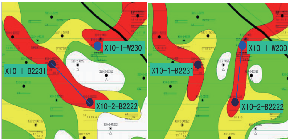
Figure 6 Facies Map Before (a) and After (b) the Combination of Well Logging and Seismic of PI2 1b
