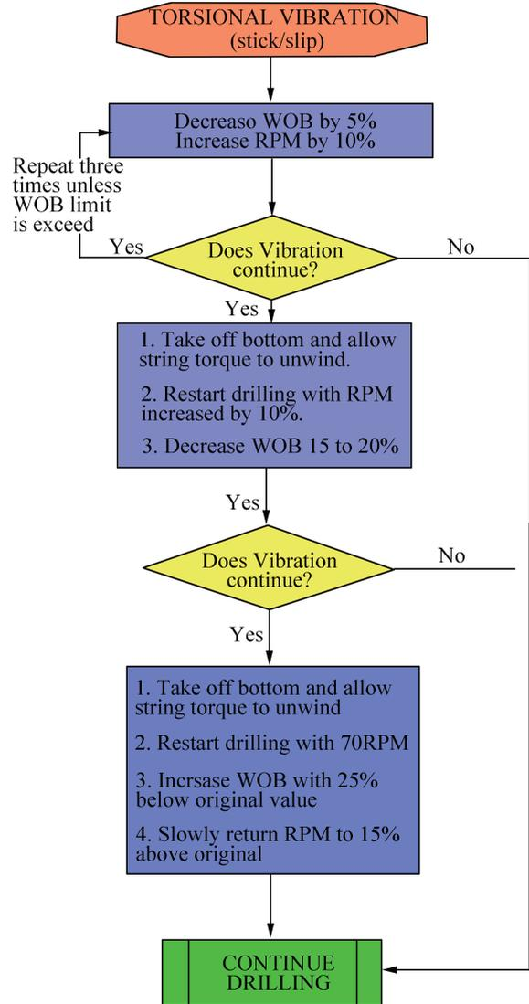
Figure 3 The Structured Method for Stick/Slip Mitigation
