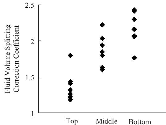
**Figure 3 Correction Charts of Fluid Splitting in Water-Flooded Wells and Layers**
