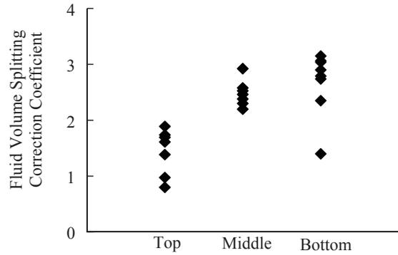
**Figure 2 Correction Charts of Fluid Splitting in Coring Wells and Layers**
