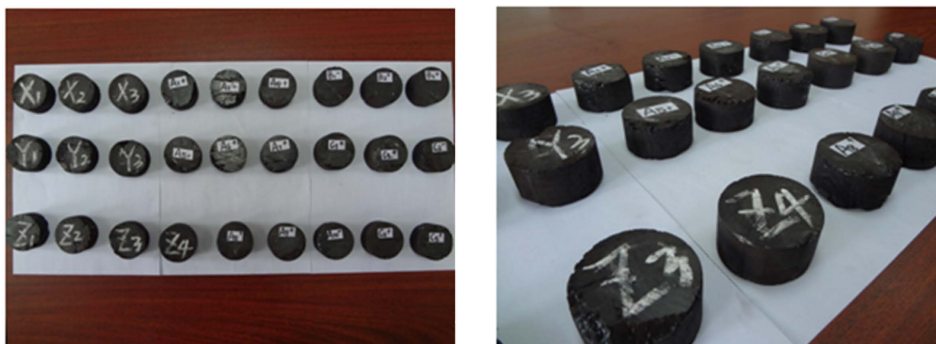
Figure 2 The Coal Sample of Tension Test and Shear Test ( \Phi 50 mm)
