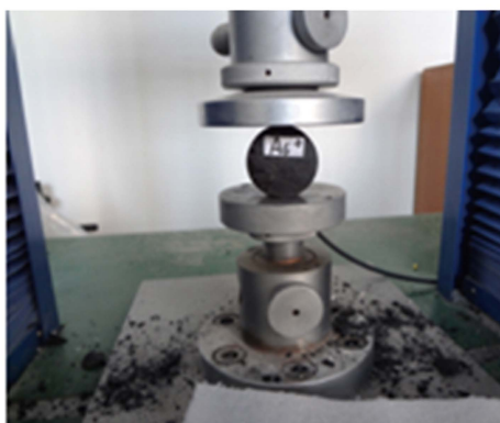
(a) The Loading Process of Coal Sample A6
