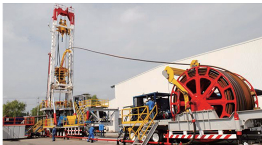
Figure 1 Slim Hole Coiled Tubing Drilling System
